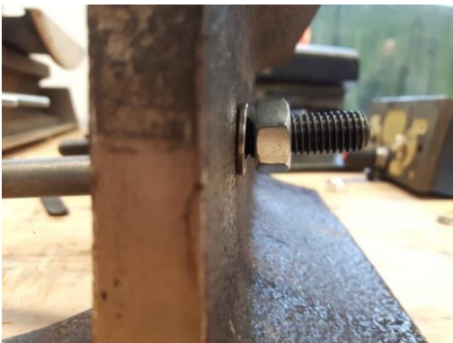
Illustration 28: Mounted eccentric screw
