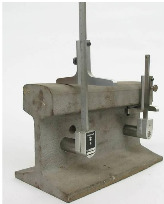
Illustration 18: Checking the drilling distances with SBKL (right) or SAHL 1 (left)
