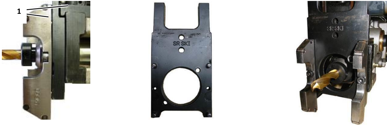
Illustration 7: Mounted jaw profiles and drills on the base plate
