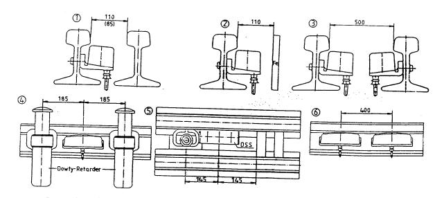
If the installation dimensions are arranged favorably, changes in the height of the wheel cannot destroy the switch
